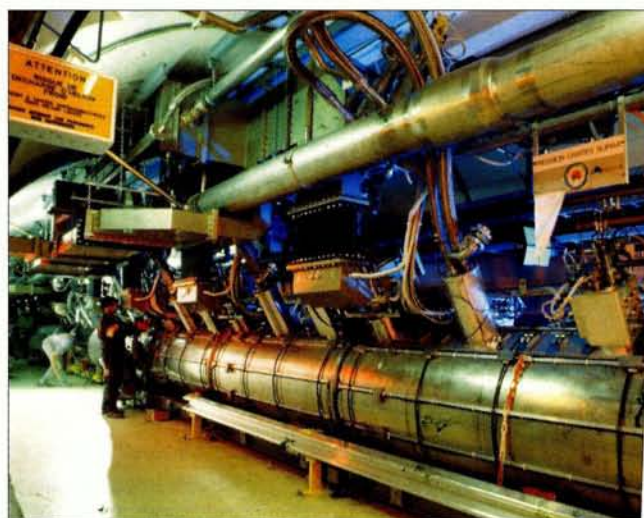
Fig. 5. One of the first of the 288 superconducting radio-frequency modules, which was installed to eventually double the energy of the Large Electron-Positron collider.
