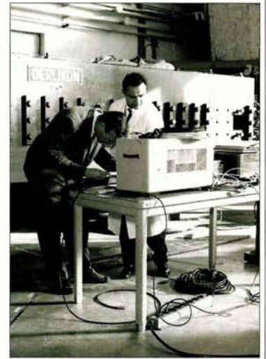
Fig. 4. Farley (left) and Zichichi pictured working on magnetic measurements and shimming.
