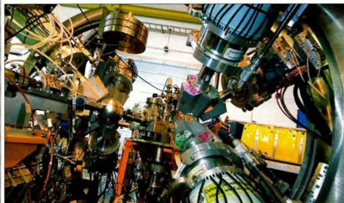
The Miniball set-up at the REX-ISOLDE facility for studying the spectra of exotic short-lived nuclei.
