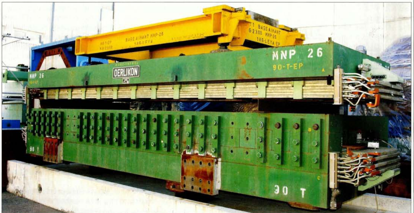
Fig. 5. The first g-2 magnet now retired at CERN; disassembled but still on site and, perhaps, ready to become an historical exhibit.
